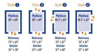
Our 4 standard platform configurations are designed to suit most applications. However, The Victorian can be custom designed to accommodate any unique accessibility needs.
